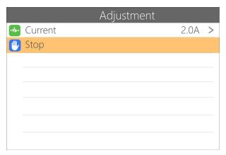
To end the charging and discharging work, short press [Scroll Wheel], move the cursor to [Stop], short press [Scroll Wheel], stop working and return to the main interface.
