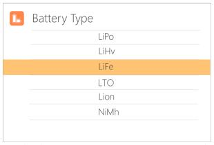
The charger supports Lipo, LiHV, LiFe, Lion, NiMh, PB chemistry batteries. After choosing the correct battery type, Short press [OK] and [CH/Exit] to take effect, and return to the previous interface.
